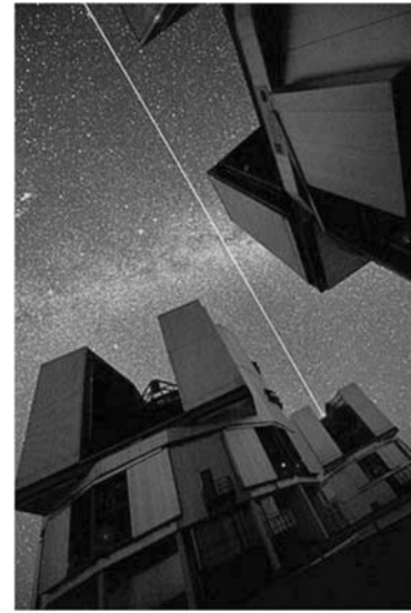
Fig. 23 The laser beam, launched from VLT's 8.2-metre Yepun telescope, crosses the sky and creates an artificial star at 90 km altitude in the high Earth's mesosphere. Notice that the spreading of the beam is extremely small. [Photograph by Dr. G Huedepohl. The photograph (in the public domain) is adapted from http://www.eso.org/public/images/gerd_huedepohl_4/ ].
