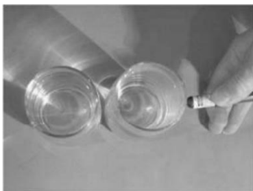
Fig. 12 The glass on the right contains distilled water and the glass on the left glass contains distilled water with few drops of milk. Because of scattering, the laser beam can be easily seen as it traverses through the liquid. Figure adapted from http://silver-lightning.com/tyndall/ . [The Photograph was taken by Mr. Marshall Dudley; used with kind permission from Mr. Marshall Dudley].
